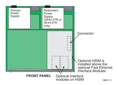
Figure C-3 Fast Ethernet Interface Module Connector Location
